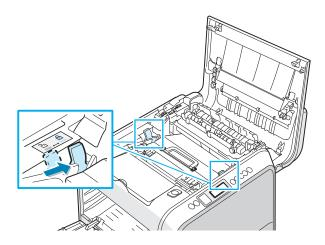
12 After making sure that the left cover is open, close the top cover. Make sure that it is securely latched.
